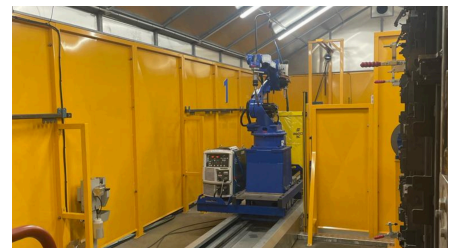
Yaskawa AR3120 robot on a 4m linear track.
