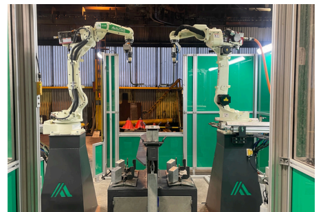
Dual Autoa welding robots awaiting next yoke.
