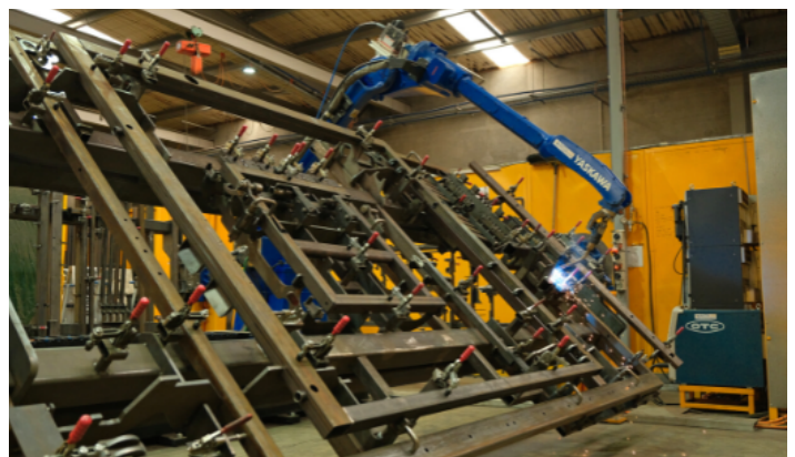
Yaskawa AR3120 robot welding livestock handling components.
