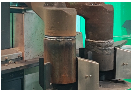
Finished weld result, between 7-9 passes, full penetration.
