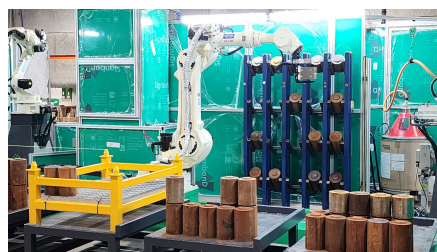
OTC V100 Handling Robot Managing Yoke Storage and Positioning.
