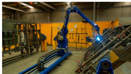
Robotic welding cell with servo-driven track.
