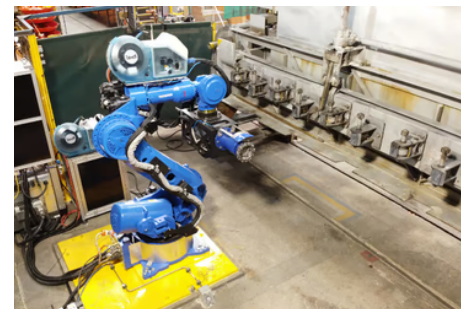
Autoa welding robot awaiting next super structure.
