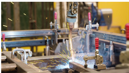
Precision MIG welding with custom jig fixtures.
