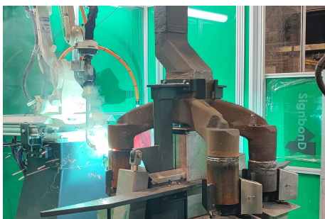
Autoa welding robot in action, repairing a stub.
