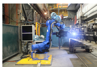
Autoa welding robot in action, repairing a super structure.
